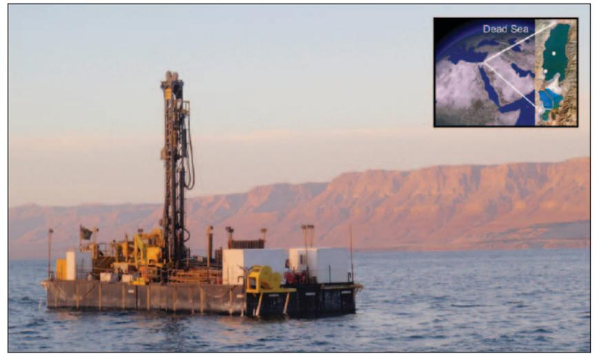
Fig. 1. The Drilling, Observation and Sampling of the Earth's Continental Crust, Inc. (DOSECC), drilling rig in the Dead Sea, drilling at a water depth of 300 meters. Inset shows locations of the drill sites in the Dead Sea (white circles). The map illustrates the location of the Dead Sea Basin, in between the Arabian-Sahara desert belt and the Mediterranean climate zone.
